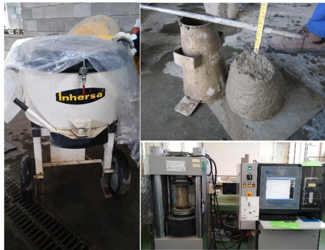
Figure 3. Images of planetary concrete mixer, slump test and compression test. Source: own elaboration.
