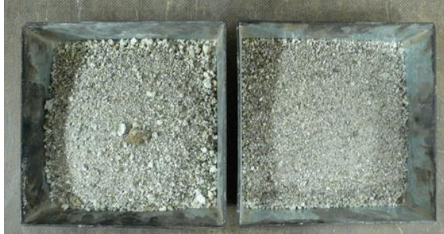
Figure 1. Slags from the stockpile before and after being tamped down. Source: Personal compilation, 2014.
