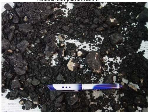
Figure 2. Marshall specimen of mixture AC32-Base G shredded after compaction. Source: Personal compilation, 2014.
